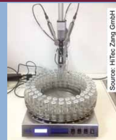
Figure 3: Automated micro gas test
